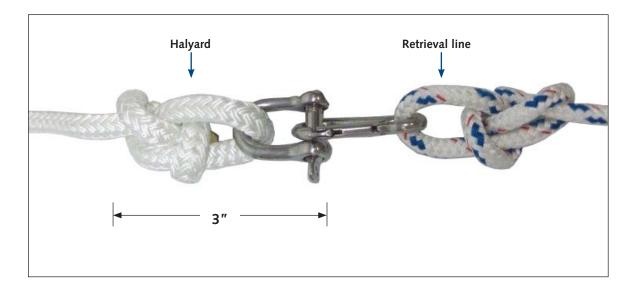
Record this measurement on the Internal Luff Groove Order Form - Line E.
