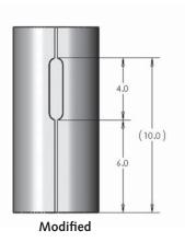
If your current mast gate configuration does not meet the above parameters, you will have to modify your existing mast gate accordingly.
