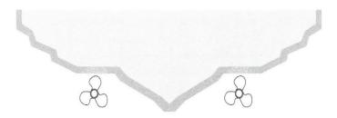
**Type Two:** Molds which require modification to achieve a "flat" surface or pocket to accept a standard FRP tube.
