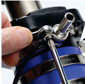
Attaching Sensor to fitting (water hose removed for photo)
